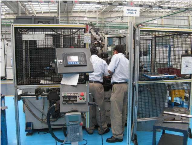
Prolonged access to hazardous cell
