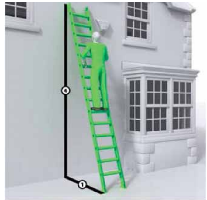
Figure 1 Ladder showing the correct 1 in 4 angle (means of securing omitted for clarity)
