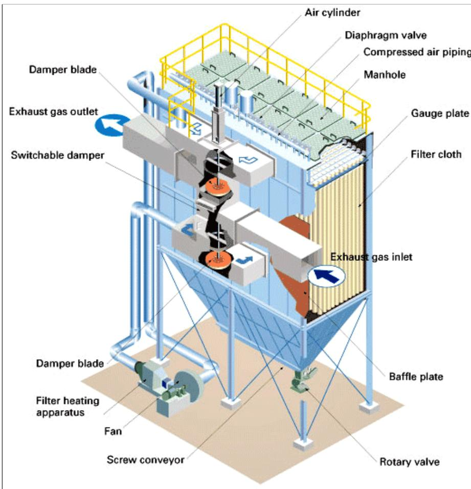
The large filtration unit, shown on the left, is a very sophisticated design, capable of dealing with large volumes of contaminant, a range of ambient temperatures and includes provision for appropriate cleaning /maintenance procedures. It would normally be located outside a building to reduce noise within the working area and to
