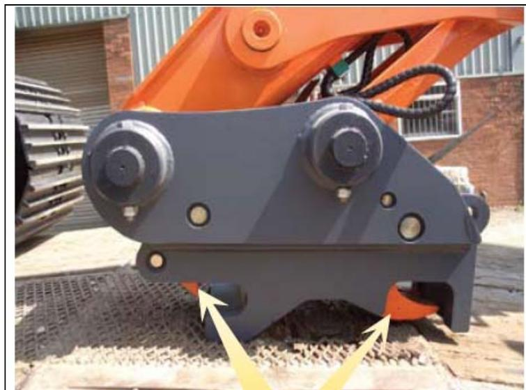
Hydraulically operated pivot pin retaining mechanisms (in orange)- the hydraulic hose connections can be seen at the top of the picture.
