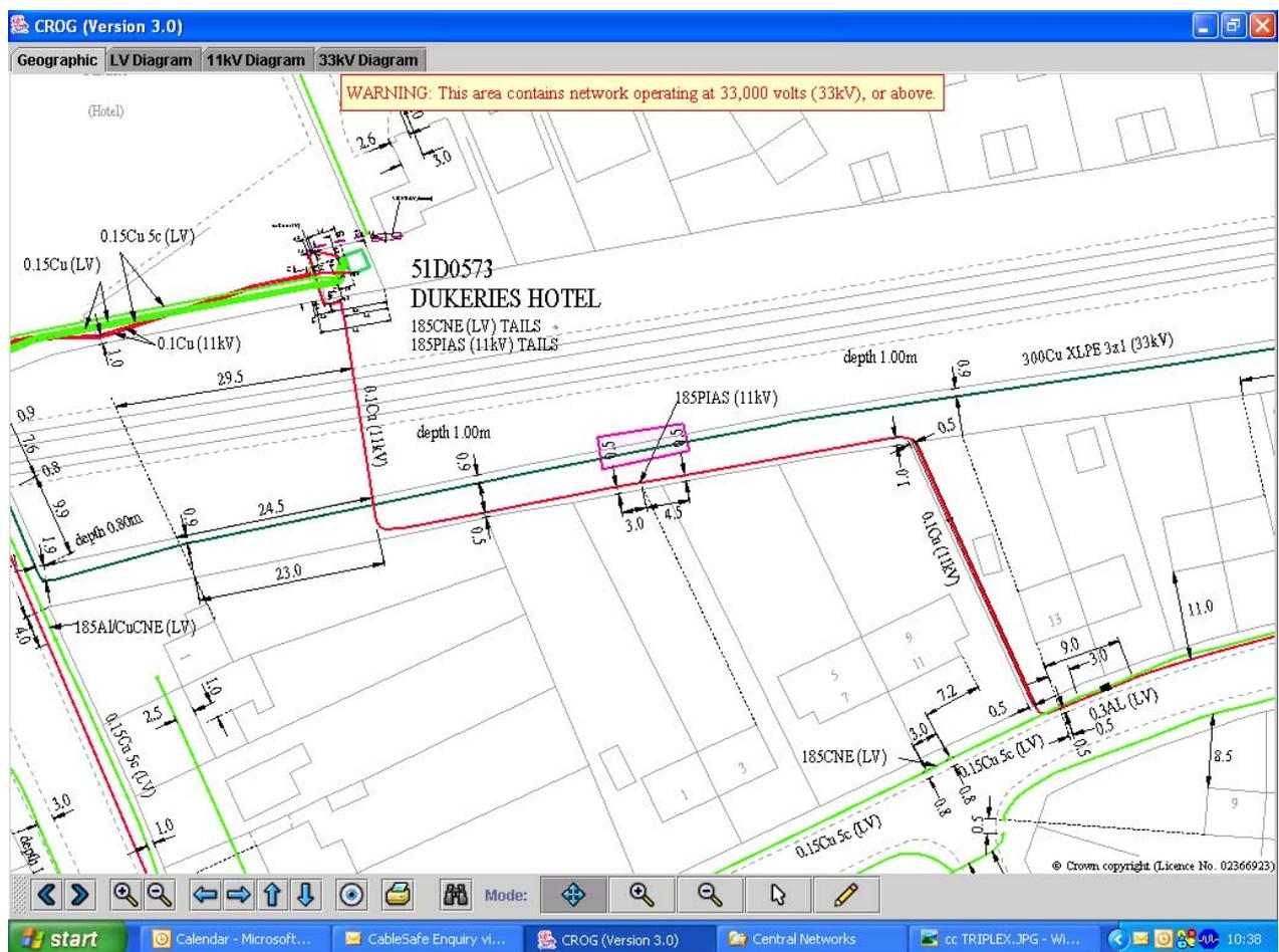
**Typical underground electrical system plans. Scale 1:500**
