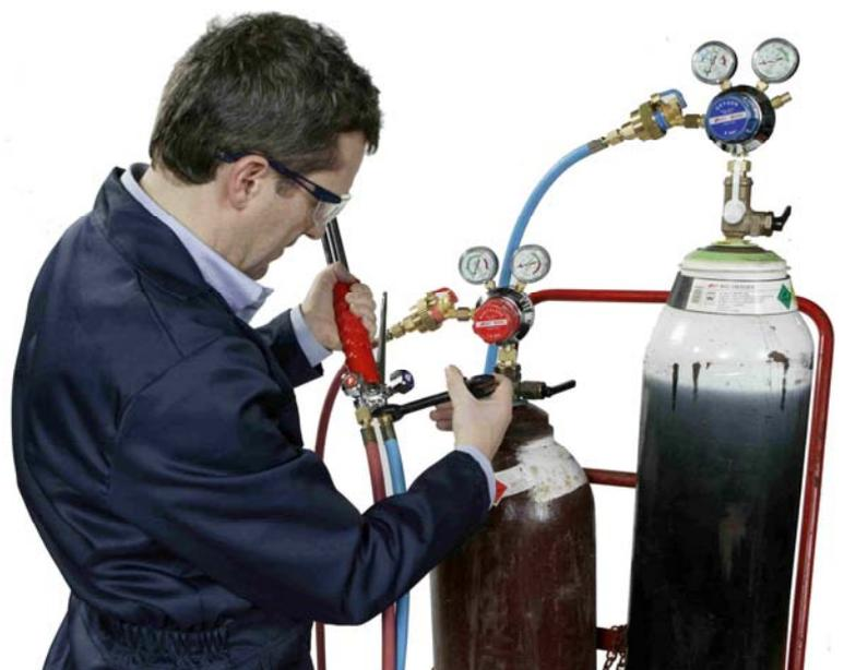
Colour-coded pipes on an Oxy-Acetylene rig
