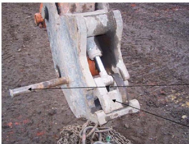
Photo 1: Semi-automatic type of QH (Safety pin about to be inserted)
